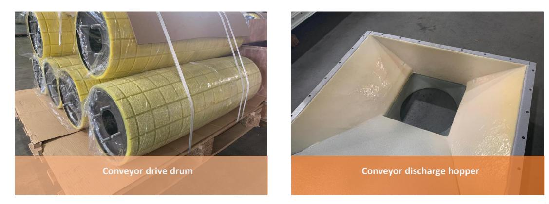
Polymer coatings have been used successfully for years to extend the life of machines and parts, including in the shipbuilding, mining, construction, energy and petrochemical industries.
