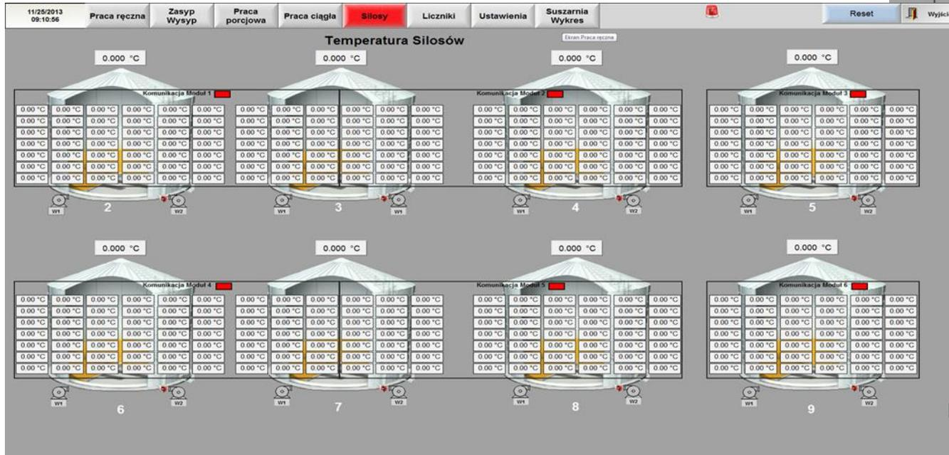
The readout is possible with the help of the object control application which allows automatic control of ventilation inside the silos and enables data archiving. In the case of a small number of probes, we can use a portable terminal, from which we can read up to two probes from one module.
